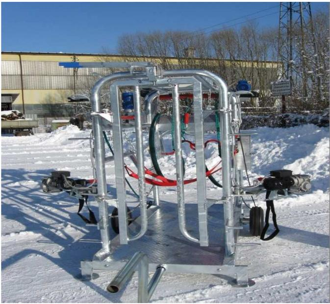
Self-locking head gate and a set of pumped wheels, an axis and a drawbar for hand transport
