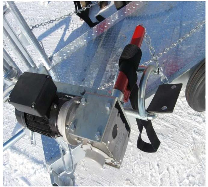
Electric front leg lifts with rubber front hoof support set with a chain enabling hooves adjustments
